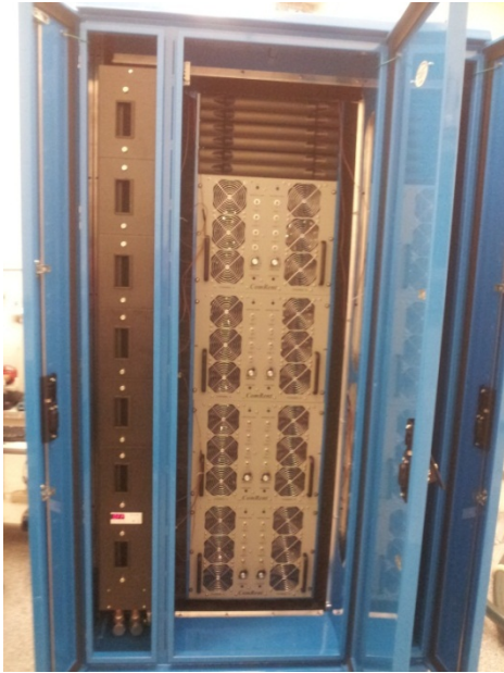
R.A.S.E.R. HD 44Kw of Load Bank
